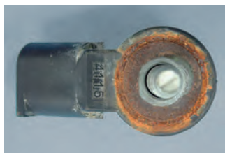
②座面の錆
